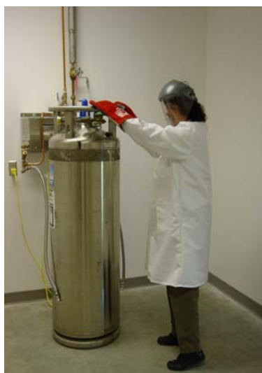
Pictured above: Carla Ramirez venting a Nitrogen tank
